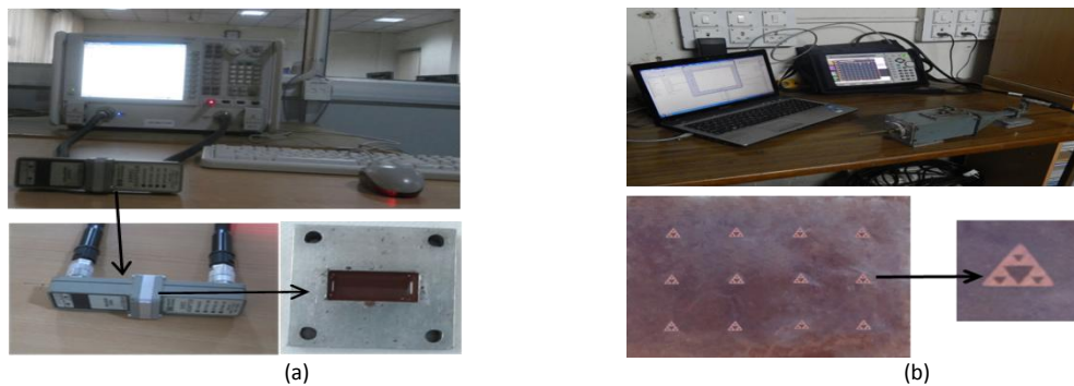
Fig. Experimental measurement setup (a) transmission-reflection waveguide setup with measured sample and, (b) ATD setup with fractal FSS embedded sample.
