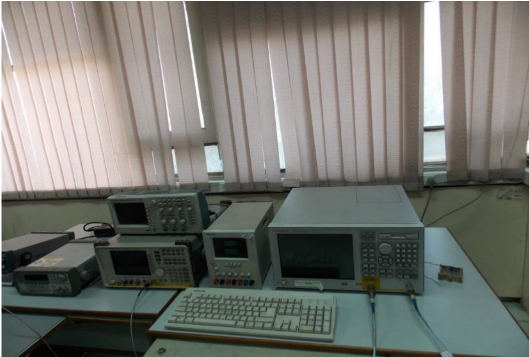
iii. General Measurement setup having Agilent VNA upto 26.5GHz, Agilent spectrum Analyzer upto 40GHz and power supplies
