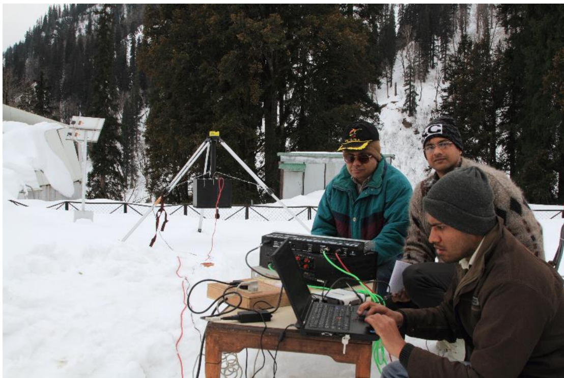
Acoustic Reflectometry System developed in CARE in use in field studies at Dhundi for determination of structure of snow layers and determination of snow water equivalent
