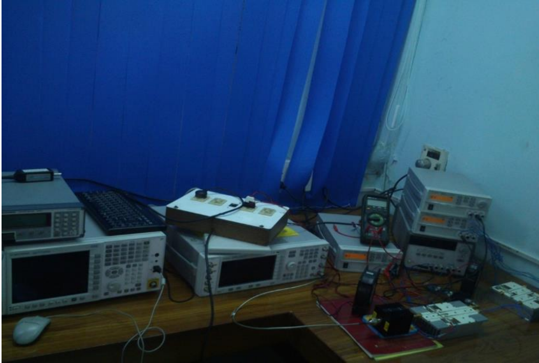
iii. Measurement setup characterizing for Non-Linearity & Digital Pre-Distortion
