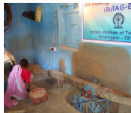
Motorized dhenki at Govindpur
