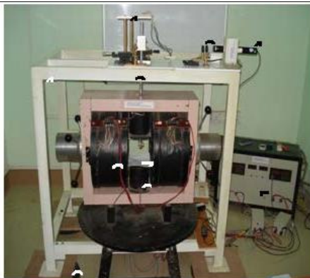
Home made cantilever beam magnetometer (CBM) in MTech teaching laboratory of our department.
