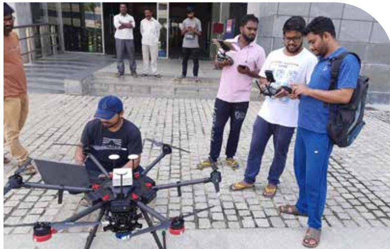
Fig: (right) Lidar mounted on UAV (left) Lidar point cloud
