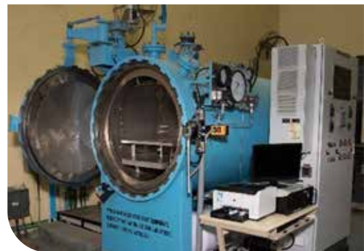
Autoclave System for Composite Manufacturing
