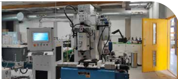
Ultrasonic C-scan immersion, Phased array, and Air-coupled systems
