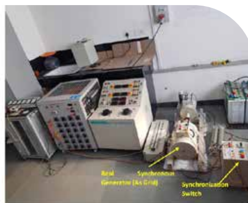
Another view of laboratory test setup for synchronizing Inverter with DC motor driven SS made for islanded and grid connected mode of operations.
