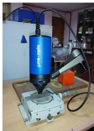
Optosurf sensor for surface quality measurement
