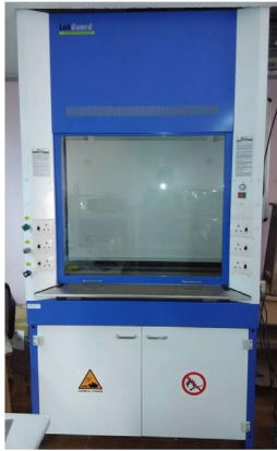
Fume hood for joint preparation
