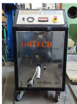
Dry ice blasting for surface cleaning
