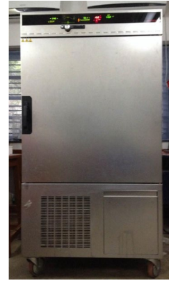
Controlled environmental chamber for ageing studies
