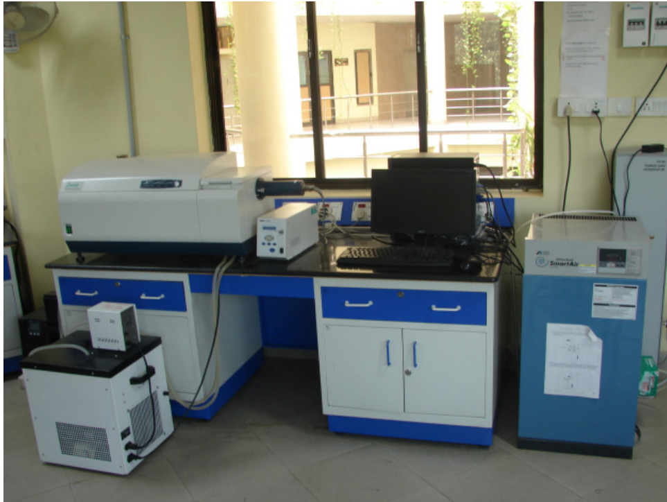
CD (Circular dichroism) Spectrometer : Used for estimation of protein and nucleic acid conformation (secondary and tertiary structure). Determination of conformational changes due to the interactions of molecule with the protein
