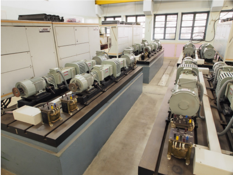
State-of-the-art Machines Lab, which has 40 sets of machines, each of which can handle almost all AC and DC machine experiments
