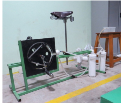
Sustainable Manufacturing Laboratory: Pedal Powered Water Filtration System
