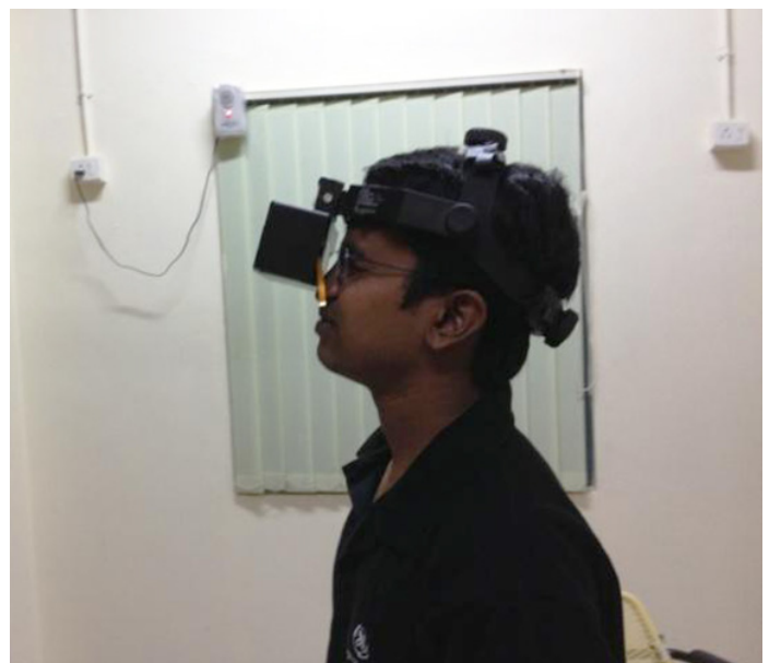
A vision aid that uses optical diffractive elements to help increase field of view for those with vision problems
