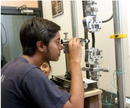
Materials and Design Laboratory: Fatigue test rated 15 kN UTM
