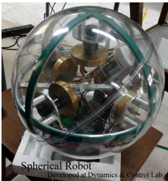
A spherical robot that can navigate stably over uneven terrain
