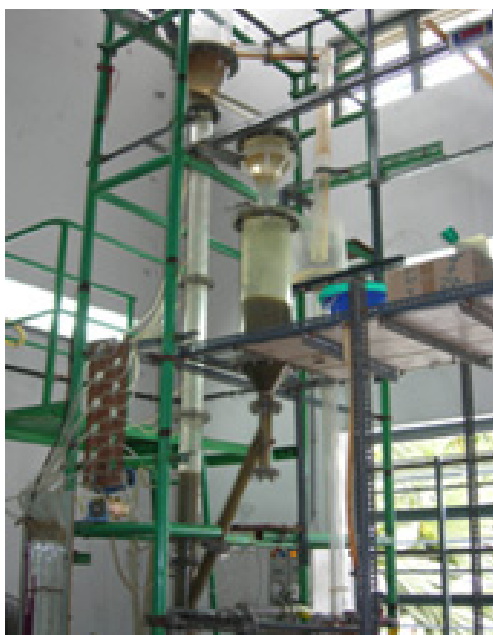
This micro pilot plant equipment is designed and fabricated in Chemical engineering Department. It is used to obtain hydrodynamic information which is required for the design of large scale commercial plants.
