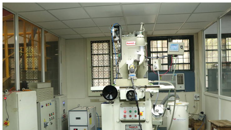
1. High-speed superabrasive grinding facility for miniature wheels located at Machine Tool Lab, Central Workshop.
