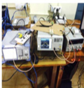
A prototype for in-band full duplex radios using off the shelf RF components
