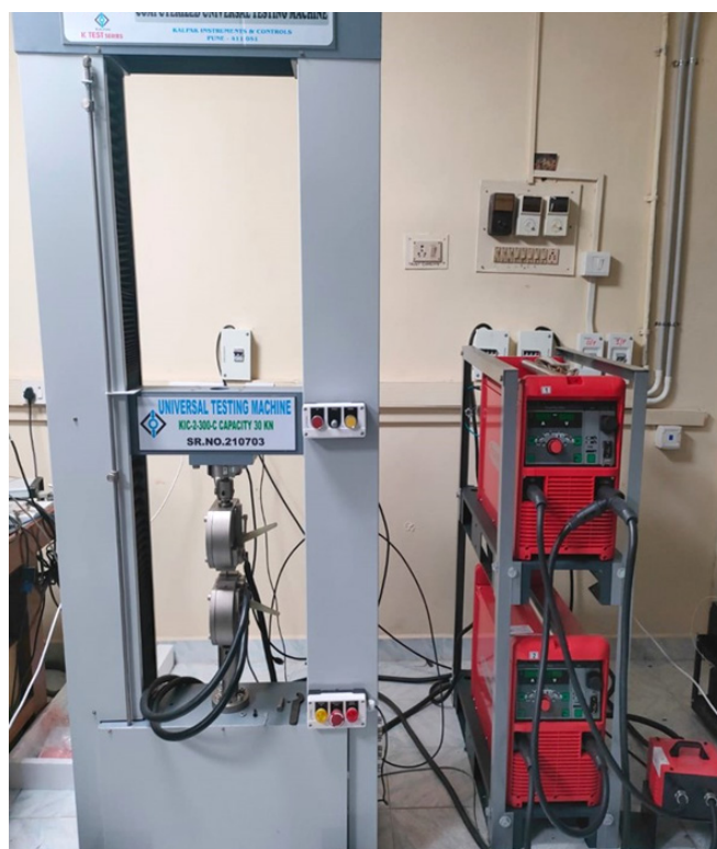
Universal testing machine with DC power source for electrical-assisted uniaxial deformation.
