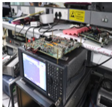
A prototype for in-band full duplex radios using off the shelf RF components
