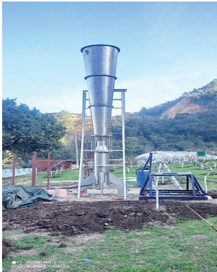
Anti-Hail Gun installation at KVK Kandaghat, Solan, HP
