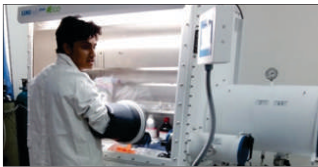
Glove box for battery research: Mbraun UniLab
