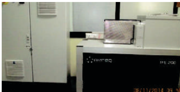
Equipment: TFS 200, BENEQ: Atomic Layer Deposition (ALD), as a thin film coating method.
