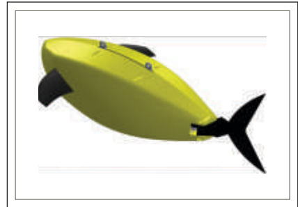
Design of Hybrid Underwater Vehicle with fin propulsion
