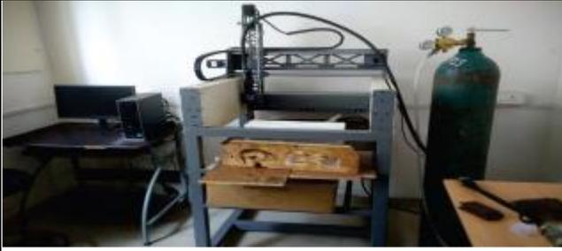
GMAW based Wire Arc Additive Manufacturing
