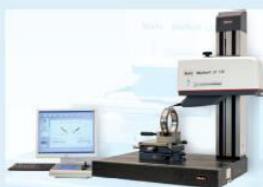
1. 3D Surface Roughness Measuring-cum-Contour Tracing Equipment (Model: LD 130 from Mahr Germany): Procured and installed
