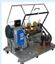
7. Machinery Fault Simulator (Model: MFS 2010 PK-7 from Spectraquest Inc. USA): Procured and installed
