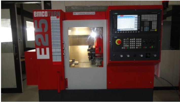
CNC Turning Center : EMCOTURN E 25 with Sinumerik 828D controller
