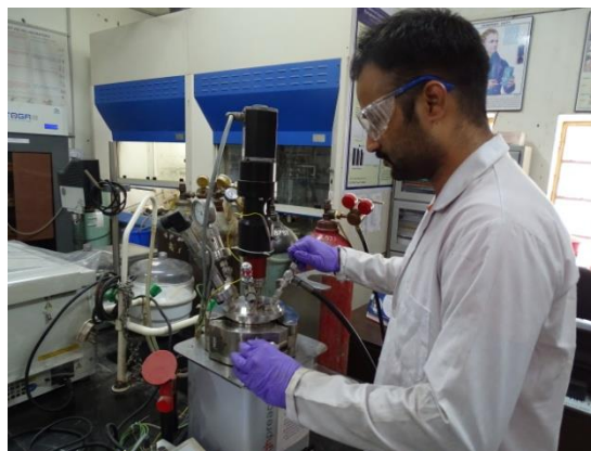
High Pressure Reactor
