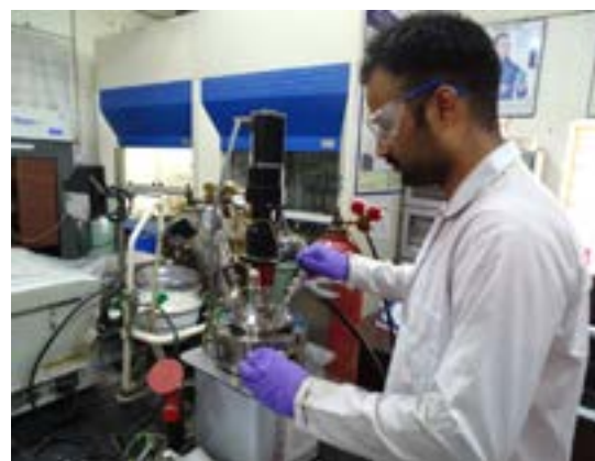
High Pressure Reactor
