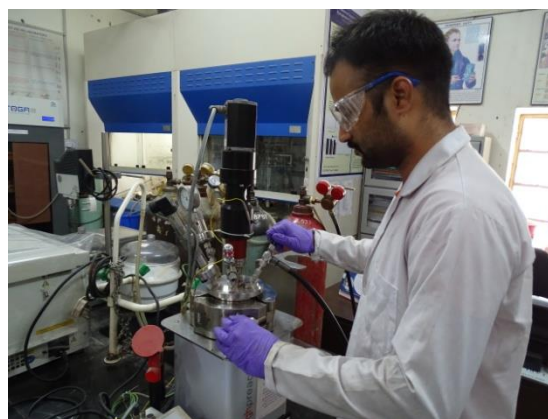
High Pressure Reactor
